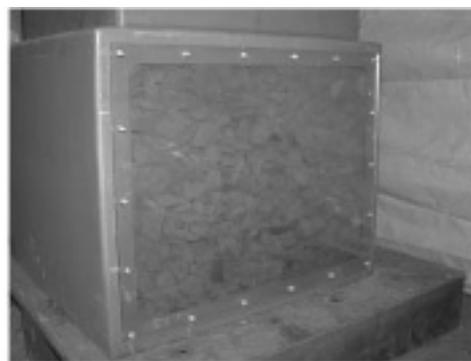
Fig.18 Filling of crushed graphite into containers by remote handling
