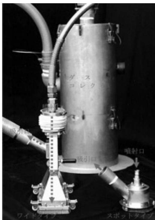
Fig.8 Suction Type Dry Ice Blast System
